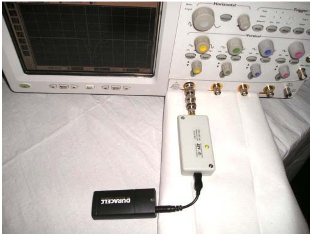
Figure 2. Test Setup With Charger and Comb Generator
