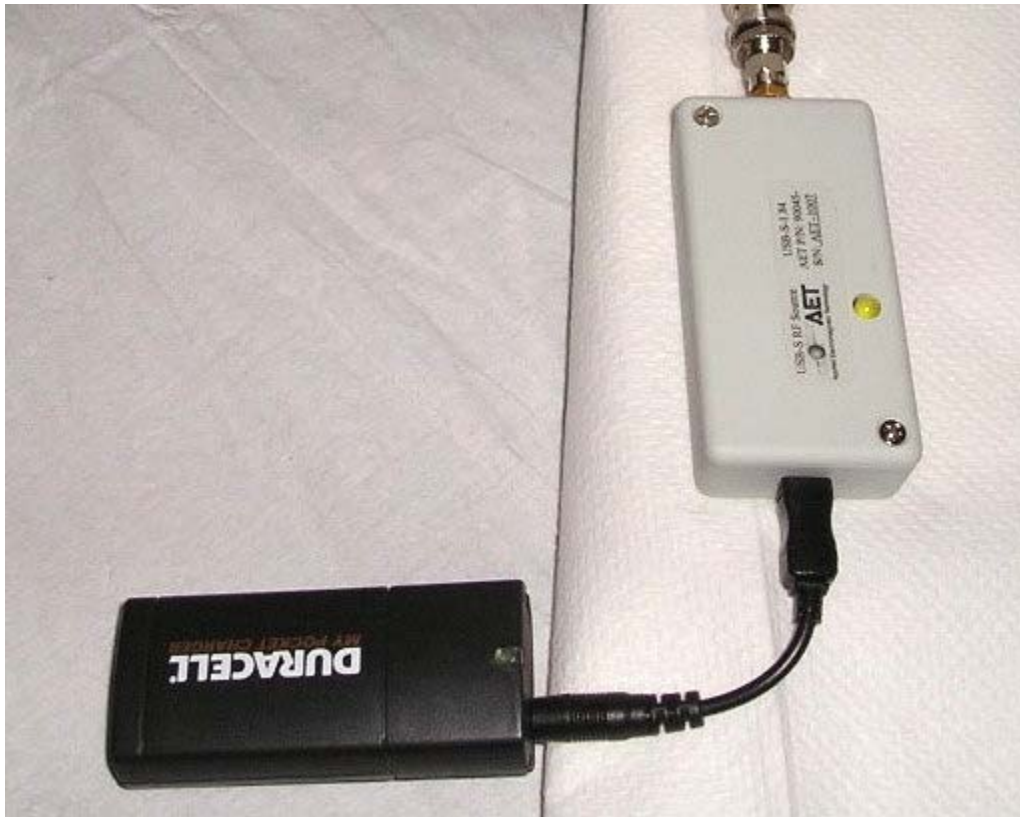
Figure 3. Close-up of Power Source and Comb Generator
