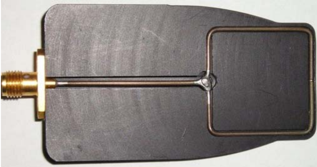
Figure 2. Construction of a Square Shielded Loop
